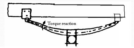
When the spring deflects in the manner bevel pinion shaft will change its position.
